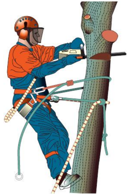
Section felling using spikes
